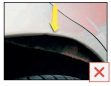
Damages of the mud protection and other exterior components.
