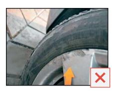
Surface deterioration on alloy wheels is not acceptable.
