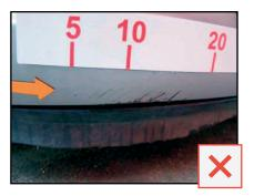
Scratches, which penetrated through to the base coat are not acceptable.
