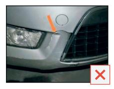
Broken, cracked or excessive damages are not acceptable.
