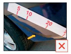
Scuffing and scratches, which penetrated through to the base coat are not acceptable. Two or more scuffs or scratches on one panel/body part are not acceptable.
