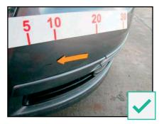
For painted bumpers - Light chipping and scratches which have not penetrated the paint coat.
