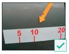
Scratches up to 90 mm are acceptable except where primer or bare metal is showing.
