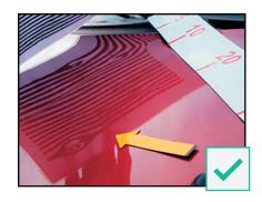
In all cases, damage greater than 20 mm is unacceptable, therefore this dent is acceptable as it is clearly with in the 20 mm tolerance.
