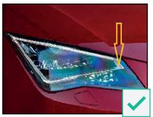
Small stone chips (not parking scrathes) on the headlights, which do not affect the light beam and are under 4 mm of size.
