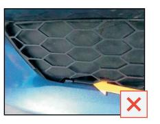
Broken, cracked grille is not acceptable.
