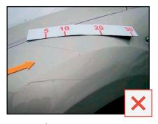
Scratches/multiple scratches or abrasions which (relative to age and Mileage) are over 100 mm in length, have penetrated the paint and cannot be removed via mechanical polishing.
