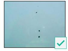
Small areas of chipping are acceptable if there is no corrosion present. Up to 3 chips per element each not larger than 3 mm.
